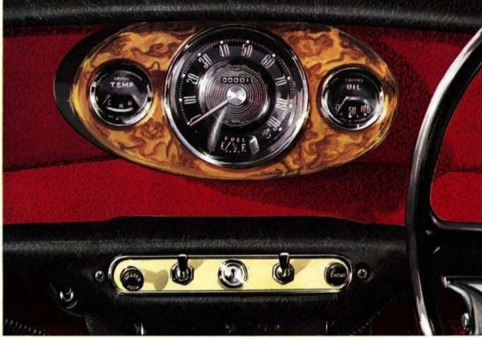
The fascia panel contains a comprehensive selection of instruments grouped in a symmetrical three-dial arrangement. The large speedometer and mileage recorder contains a fuel gauge. The two smaller dials show water temperature and engine oil pressure. There are warning lights for ignition, oil filter renewal, and headlamp main-beam. Positive-action toggle switches control the lights, and a key switch opens or closes the ignition circuit and operates the starter solenoid switch.
