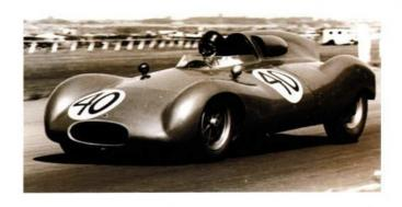
Other successful Cooper sports cars included the highly-acclaimed 'Monaco' and the 'Bobtails', the latter which proved to be yet another astounding sales success. Again employing the revolutionary principle of locating the engine behind the driver, this car, powered by a modified Coventry Climax fire-pump engine, dominated its class.
