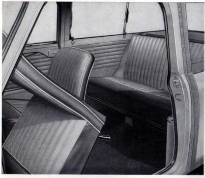
The two front seats are independently adjustable on slides and tilt forward to provide easy access to the rear.
