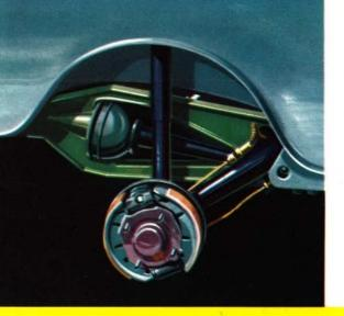
TRAILING TUBULAR levers have been employed in the independent rear suspension. The rubber 'springs' are controlled by hydraulic shock absorbers and the trailing arms carry the stub shafts for the wheel hubs. Four-wheel hydraulic brakes, with leading and trailing shoes, are controlled by pendant pedal, but for parking purposes the handbrake is mechanically connected to the rear wheels.
