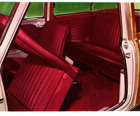
IN PRIVATE or commercial use, the interior luggage space is unrestricted. The provision of a removable cover in the rear of the floor keeps the spare wheel out of sight yet readily accessible when needed.
